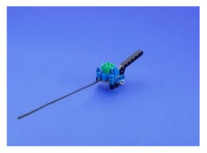
The Rear Table Sensor makes use of a Light Sensor to detect the edge of a table.
