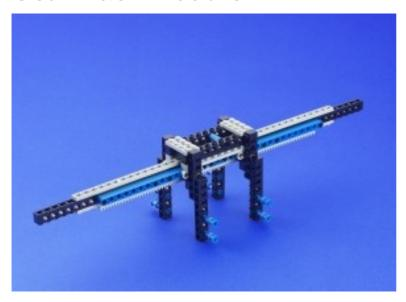
The Gear Rack Module is the overlying beam on which the Pen Module shuttles back and forth.
