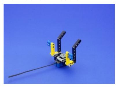
Used in both versions of the Aerial Tram this Module uses a single Light Sensor to detect either end of the Tram's overhead cable.
