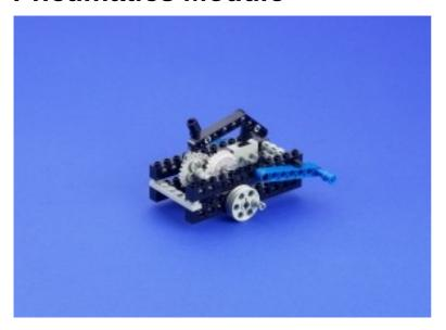
The Pneumatic Module efficiently uses one motor to both control the valve and pump air to the Pneumatic ram on the Pen Module.
