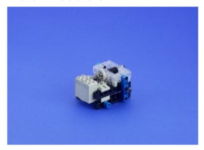
This Motor Module achieves a 24 to 1 gear ratio by transferring power from the driving axle to the output axle via a worm gear.
