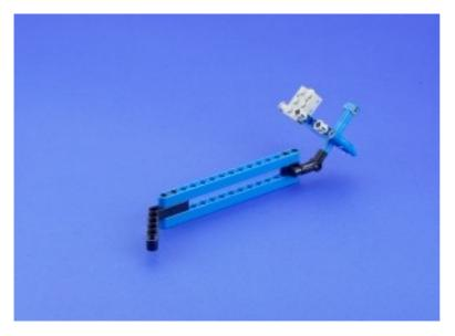
Using a simple lever mechanism the Table Sensor Module uses a Touch Sensor to detect the edge of a table.
