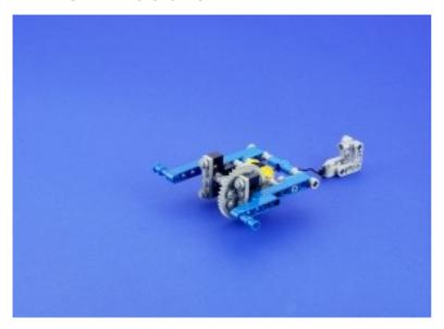
The Winch Module is designed to lower and raise a hook using a spool with a length of cable.
