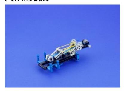
The Pen Module holds a pen in a sliding holder that is moved up and down by the Pneumatic ram.
