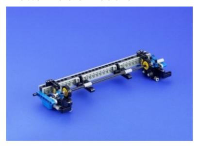
The Plotter Table Module holds a sheet of paper and can feed it back and forth via Motor Module 3.
